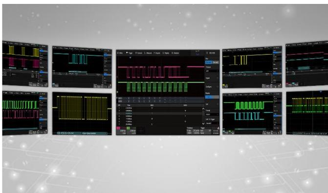
Display the decoded characters through the events list. Bus protocol information can be quickly and intuitively displayed in tabular form. I2C, SPI, UART, CAN, LIN, CAN FD, FlexRay, I2S, MIL-STD-1553B, SENT, Manchester, ARINC429 and USB 2.0 are supported
