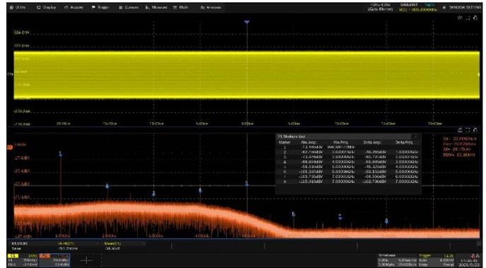
FFT supports up to 32 Mpts operation. This provides high-frequency resolution with a fast refresh rate. The FFT function also supports a variety of window functions so that it can adapt to different spectrum measurement needs. Three modes (Normal, Average, and Max hold) can satisfy different requirements for observing the power spectrum. Auto peak detection and markers are supported.
