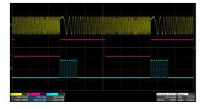
**Sweep and Burst** Sweep supports "Line" and "Log" modes, while Burst enables "NCycle" and "Gated" modes. Both Sweep and Burst support trigger sources: Internal, External, and Manual.
