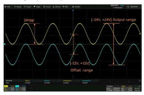
24Vpp analog output superimposed with ± 12 Vdc offset, providing a maximum output range of ± 24 V (48 V).
