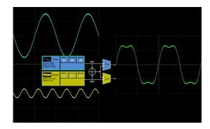
Waveform Combining Superimposes CH1 and CH2 waveforms internally and provides the combined waveform to a user-selected output. It easily combines basic waveforms, random noise, modulation signals, sweep signals, burst signals, EasyPulse waveforms, and TrueArb waveforms without external connections or complex editing.
