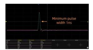
**High speed** The minimum 1 ns pulse width, can be generated at any frequency. The pulse width can be finely adjusted in steps of 10 ps.
