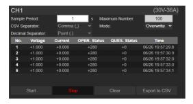
Start Button: Start data log record function.Stop Button: Stop data log record function.Clear Button: Clear data log record data.
