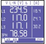
During measurements, press the **i** key to block all measurements immediately (not only those currently displayed). By doing so, the measurements will remain "frozen" on screen until the same key is pressed again.
