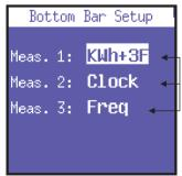
This page allows the user to choose 3 parameters (out of 63) to be displayed alternately in the bottom part of the measurement screens, in addition to the battery level. The following parameters are available for visualization:
