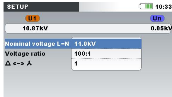
Figure 17: Voltage ratio for 11 kV / 110 kV transformer example
