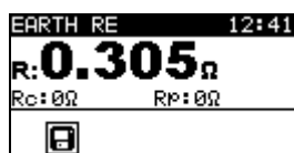
Figure 6.1: Typical display in earth resistance function
