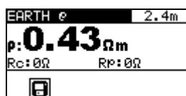
Figure 7.24: Example of specific earth resistance measurement result
