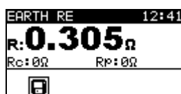
Figure 7.22: Example of earth resistance measurement result
