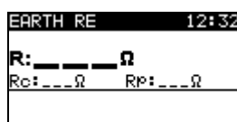
Figure 7.21: Earth resistance screen
