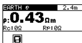
Figure 6.2: Typical display in specific earth resistance function
