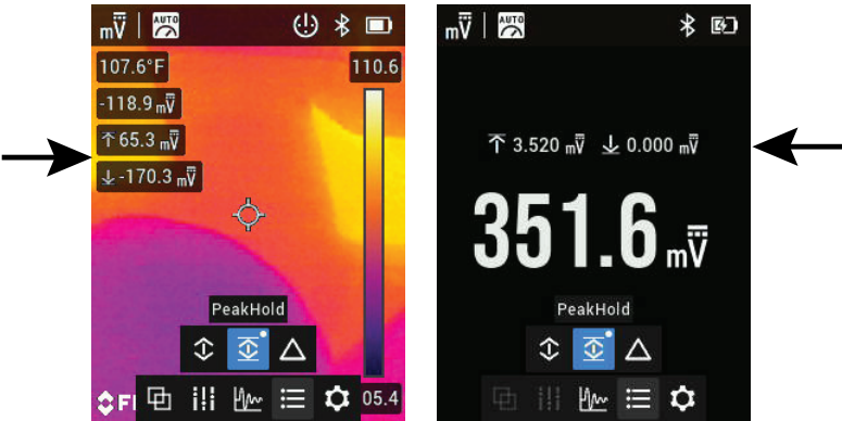
Figure 10.18 Peak Hold mode menu from the thermal image mode (left) and multimeter mode (right).
