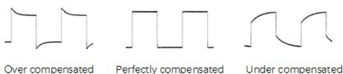
**Figure 4.9 Probe Compensation**
