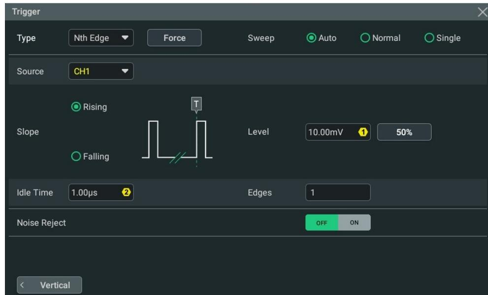
**Figure 8.23 Nth Edge Trigger Setting Menu**
