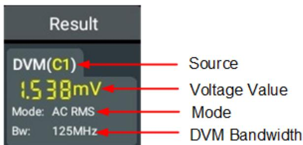
The voltage value in the label shows the measurement extrema over the last 3 seconds.
