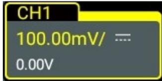
The information displayed in the channel status label is related to the current channel setting (irrelevant with the on/off status of the channel). After the channel is turned on, you can modify the parameters such as the vertical scale, horizontal time base, trigger mode, and trigger level according to the input signal for easy observation and measurement of the waveform.
