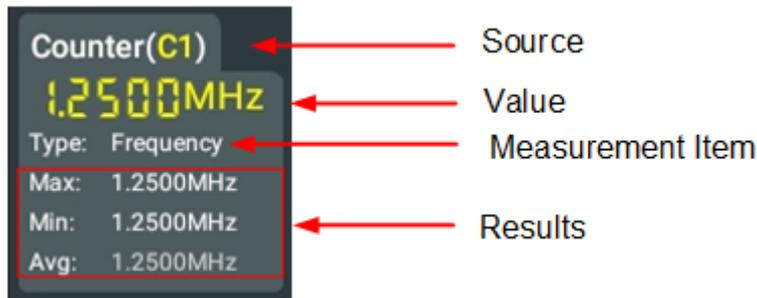
You can click or tap the "Counter" label in the "Result" bar and select **Reset Stat**, **Setting**, or **Remove** in the displayed window.
