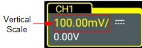
The adjustable range of the vertical scale is related to the current probe ratio. By default, the probe ratio is 1X. In this case, the adjustable range of the vertical scale is 500  $\mu$ V/div to 10 V/div.
