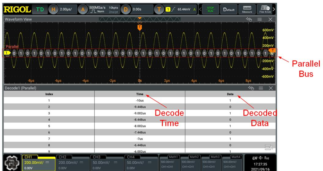
Figure 14.3 Parallel Decoding Event Table
