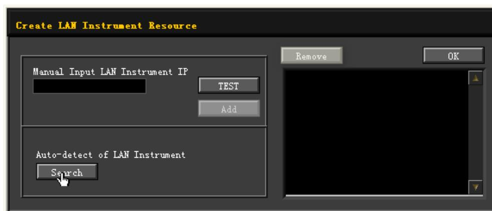
Besides, you can input the IP address of the instrument manually into the text field under "Manual Input LAN Instrument IP", then click **TEST**. If the instrument passes the test, click **ADD** to add the instrument to the LAN instrument resource list in the right section; if the instrument fails the test, please check whether the IP address that you input is correct, or use the auto search method to add the instrument resource.
