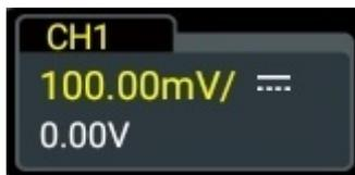
Click or tap the channel status label at the bottom of the screen or press the front-panel key
