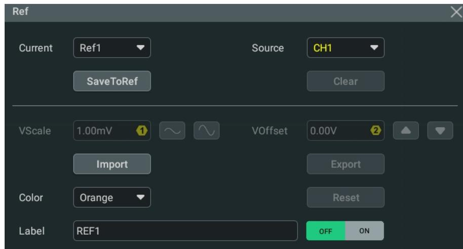
Figure 12.1 Reference Waveform Menu
