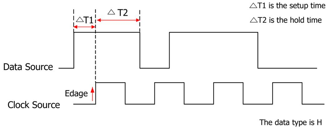
Figure 8.20 Setup/Hold Trigger
