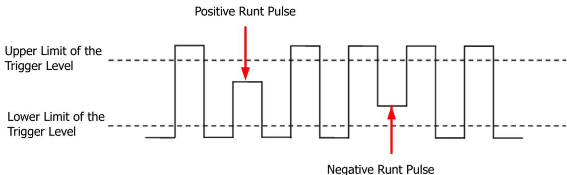
**Figure 8.15 Runt Trigger**
