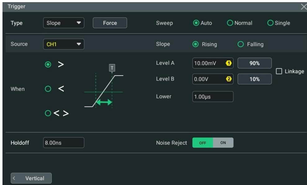
**Figure 8.7 Slope Trigger Setting Menu**
