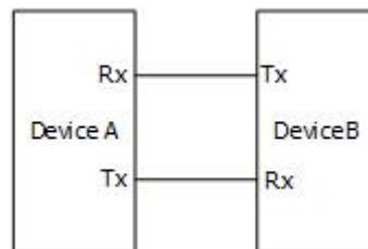
**Figure 14.4 Schematic Diagram of RS232 Serial Bus**
