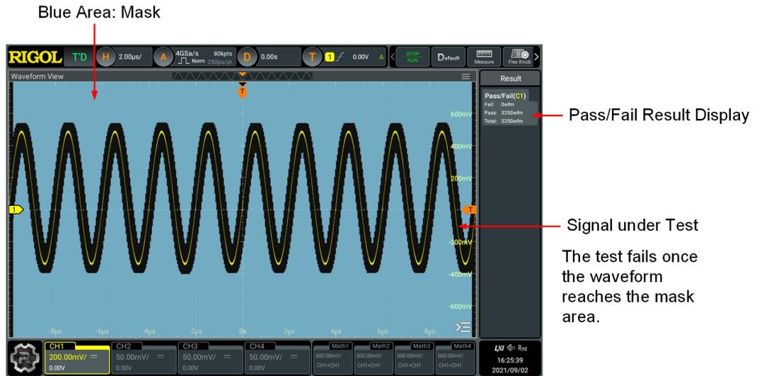
Figure 13.2 Pass/Fail Test Interface
