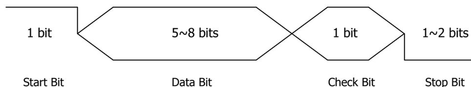
**Figure 8.24 Schematic Diagram of RS232 Protocol**
