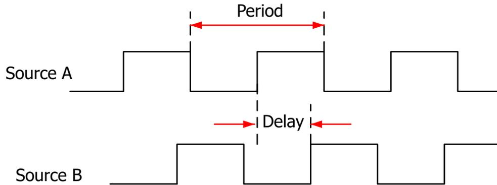
**Figure 10.2 Delay and Phase Parameters**
