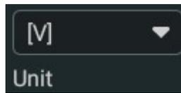
Changing the amplitude unit also changes the units of the functions related to the channel accordingly.
