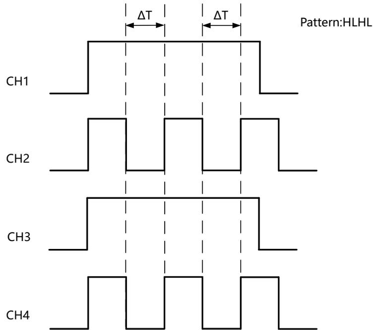
Figure 8.11 Duration Trigger
