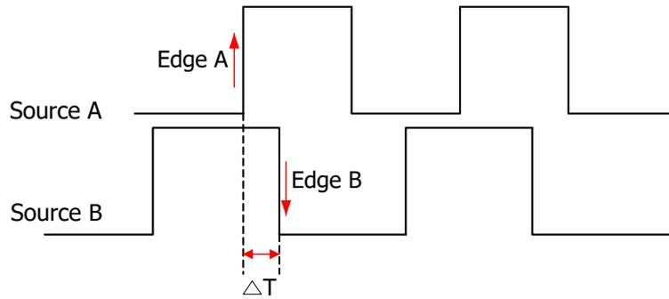
Figure 8.18 Delay Trigger
