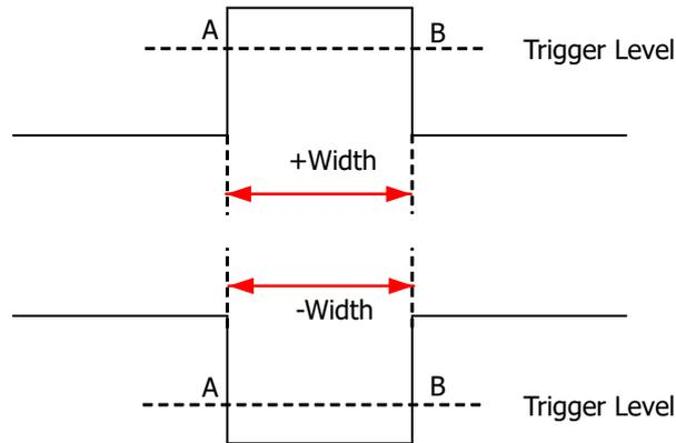
Figure 8.4 Positive/Negative Pulse Width
