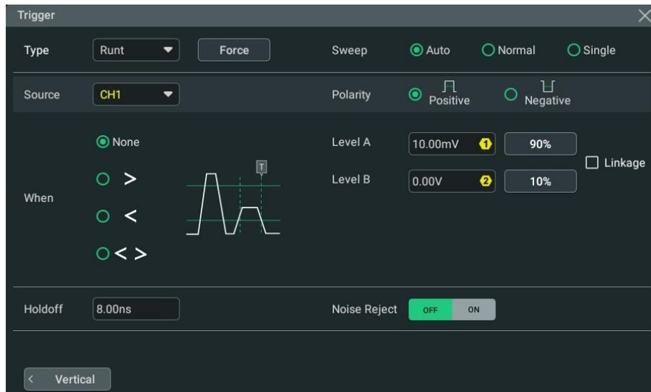
**Figure 8.16 Runt Trigger Setting Menu**
