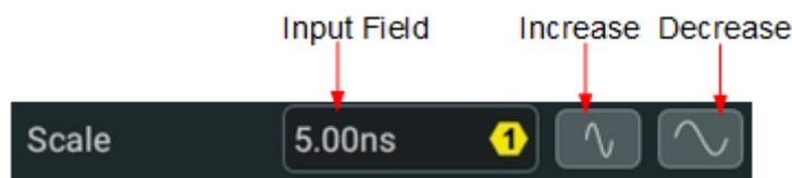
In the **Horizontal** menu, you can click or tap the **Vernier** on/off switch to toggle between ON (fine adjustment) and OFF (coarse adjustment). You can also press the
