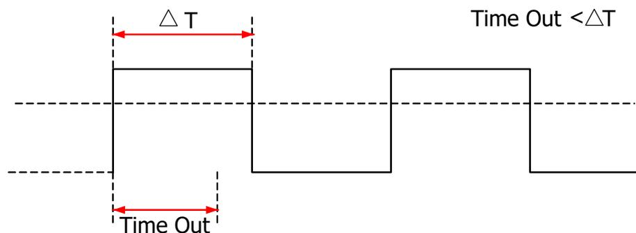
Figure 8.13 Timeout Trigger
