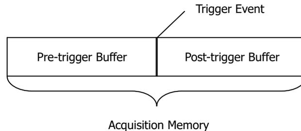
**Figure 8.1 Schematic Diagram of the Acquisition Memory**
