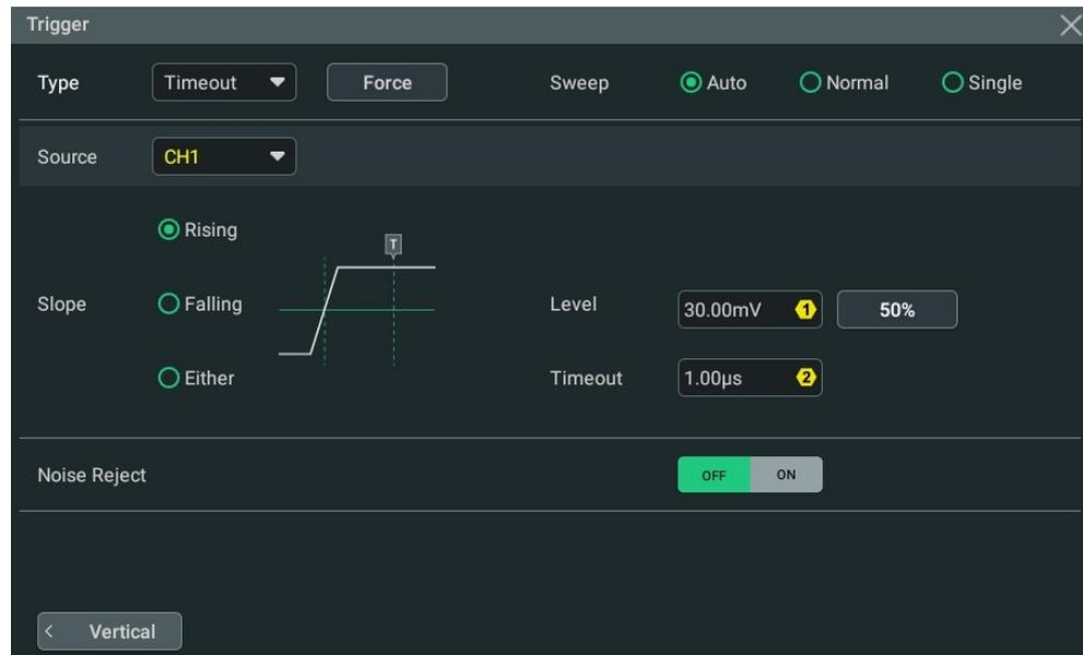
**Figure 8.14 Timeout Trigger Menu**
