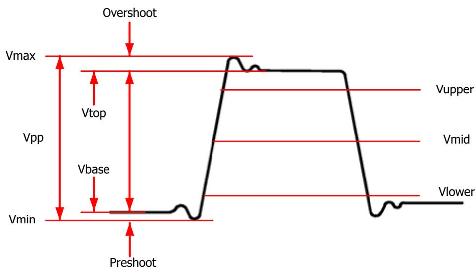
**Figure 10.3 Voltage Parameters**
