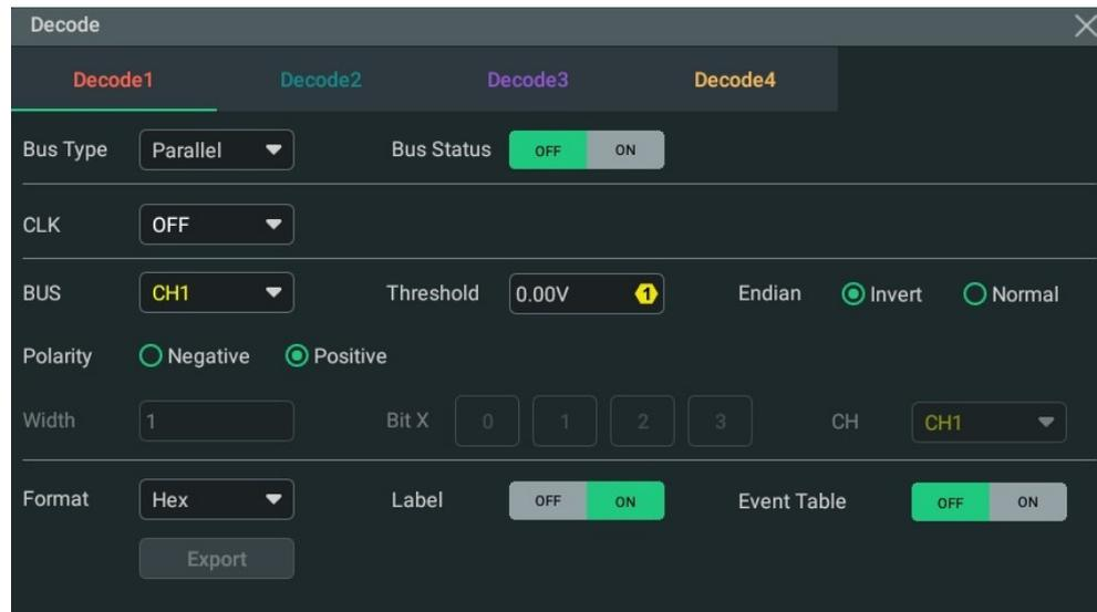
Figure 14.2 Parallel Decoding Menu
