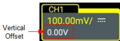
The adjustable range of the vertical offset is related to the current probe ratio and vertical scale.
