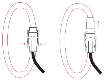
■ Close the sensor by forcing the moving part into the connector until you hear a click.
