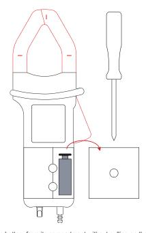
■ Withdraw the battery from its compartment without pulling on the wires.
