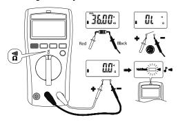
Dial the switch and press the Function button to select the measuring function.
