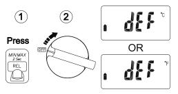
Turn on the meter after keeping the button down.
