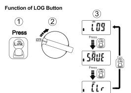
Pressing Link button while powering-up to select the mode – Data Logger mode, Manual Saving mode and Clear memory.
