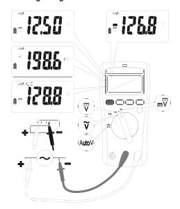
Dial the switch to select the measuring function.
