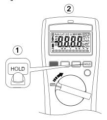
To turn on the meter after keeping HOLD button down.
