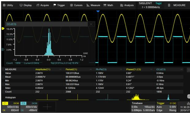
Statistics shows the current value, maximum value, minimum value, standard deviation and mean value of up to 5 parameters simultaneously. Histogram is available to show the probability distribution of a parameter.
