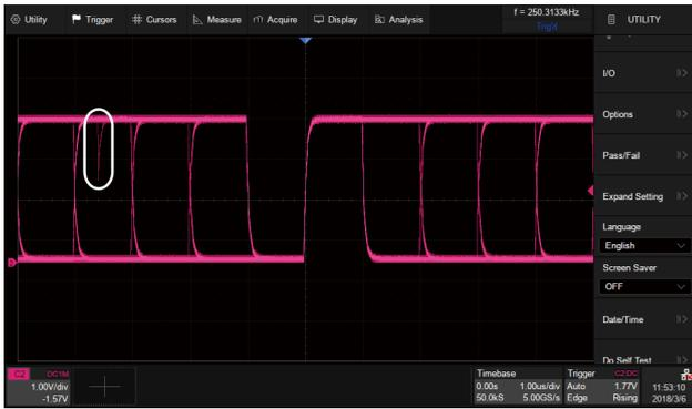
With a waveform update rate of up to 110,000 wfms/s, the oscilloscope can easily capture unusual or low-probability events. In Sequence mode the waveform capture rate can reach 480,000 wfms/s
