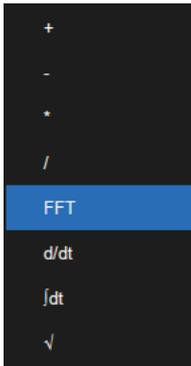
In addition to the traditional (+, -, X, /) operations, FFT, integration, differential and square root operations are supported. Math on math is available for more complex operations
