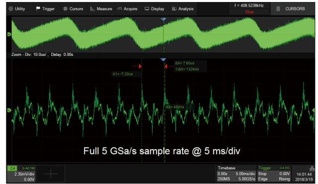
Using hardware-based Zoom technique and record length of up to 250 Mpts, users can select a slower timebase without compromising the sample rate, and then quickly zoom in to focus on the area of interest
