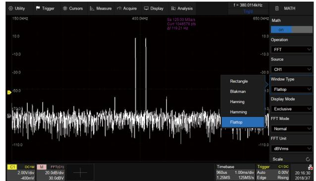
Hardware accelerated FFT supports up to 2 Mpts operation. This provides high frequency resolution with a fast refresh rate. The FFT function also supports a variety of window functions so that it can adapt to different spectrum measurement needs. Three modes (Normal, Average and Max hold) can satisfy different requirements for observing the power spectrum
