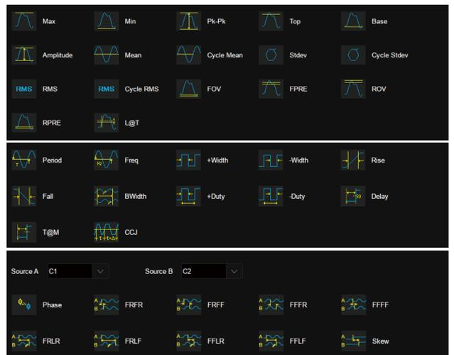
Parameter measurements includes 3 categories: horizontal, vertical and CH delay providing a total of 39 different types of measurements. Measurements can be performed within a specified gate period. Measurements on Math, Reference and History frames are supported
