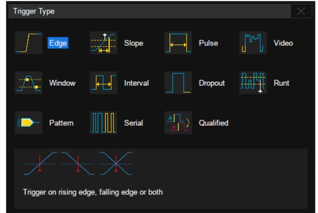
Edge, Slope, Pulse, Video, Windows, Runt, Interval, Dropout, Pattern, Qualified and serial trigger
