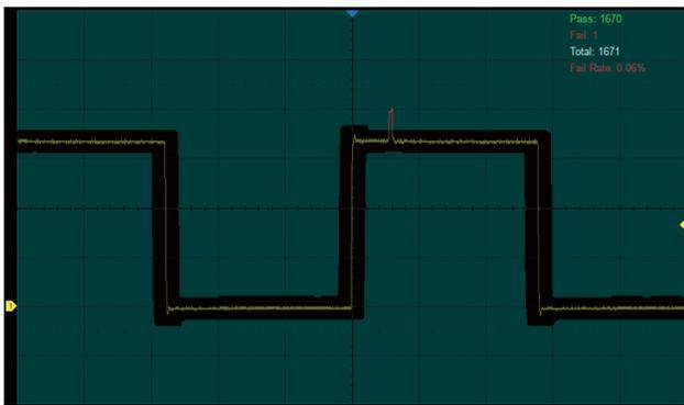
The SDS5000X utilizes a hardware-based Mask Test function, performing up to 110,000 Pass / Fail decisions each second. It is easy to generate user-defined test templates in order to provide trace mask comparisons, making it suitable for long-term signal monitoring or automated production line testing
