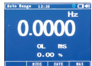
Frequency Measurement with Pulse Width and Duty Cycle
