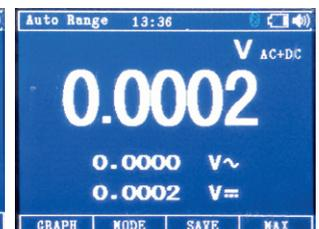
Measurement with Display for AC & DC Component Separately
