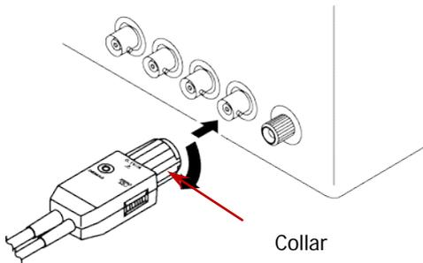
Note: When disconnecting the output connector and the measuring instrument, be sure to release the lock by rotating the collar in the opposite direction of the arrow as shown in the figure above before pulling off the connector. Forcibly pulling the connector without releasing the lock or pulling on the cable can damage the terminator.
