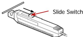
2. Align the current sensor so that the current direction indication corresponds to the direction of current flowing through the
