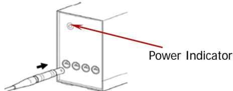
2. Turn off the power adaptor and connect it to the power supply.
