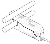
8. Be sure to use the slide switch to open the current sensor. For RP1003C and RP1004C, please do not press the upper core in the direction of the arrow as shown in the figure below to avoid damaging the internal structure of the slide switch.
