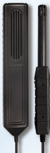
CO 2 probe Humidity/ Temp. probe
