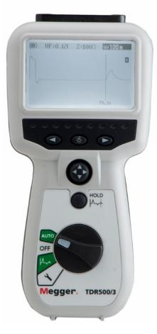
With a minimum resolution of 0.1 m and a maximum range of 5 km, these TDRs can be used on all metallic cable pairs and are ideal for a wide range of cable fault diagnostics.
