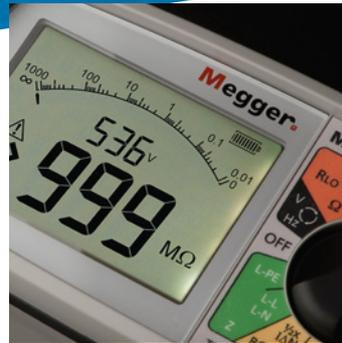
The analogue arc simulates the behaviour of a mechanical measuring needle display
