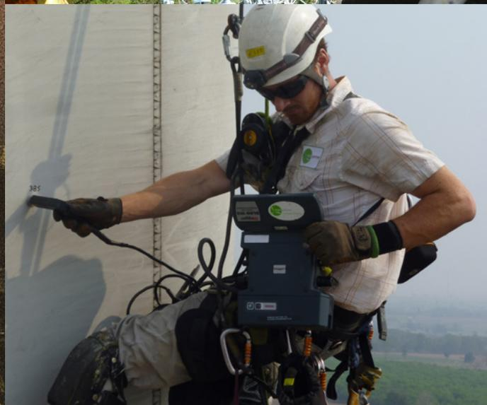
The average value is then displayed within 3 seconds, to a basic accuracy of 0.2%. DLRO 10X displays both forward and reverse measurements as well as the average of the two.
